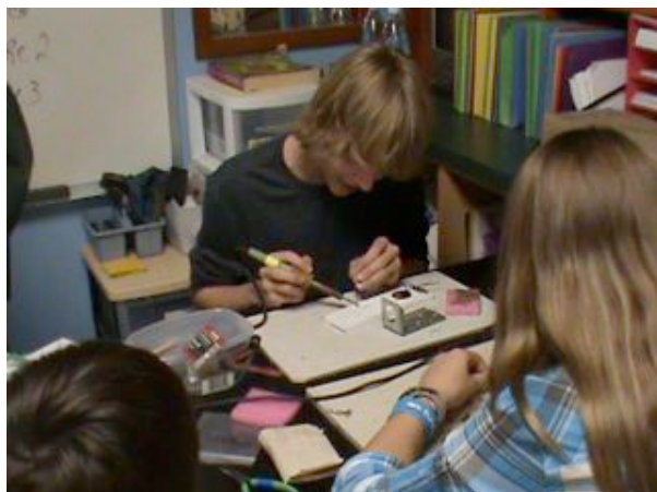
Fig. 6 Soldering lugs onto the piezoelectric sensors for connection to the output bus.
