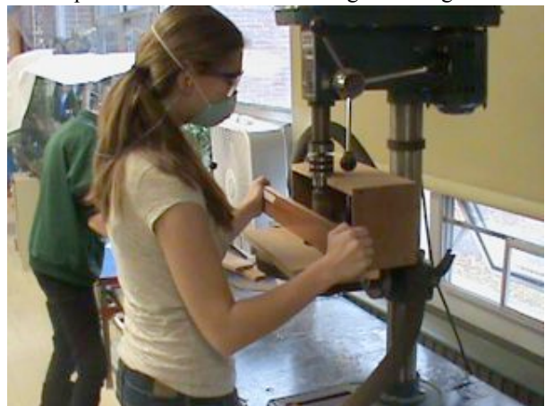
Fig. 5 Tuning by sanding the middle section of the underside of a marimba bar.
