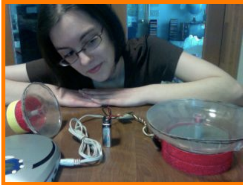
Speaker with mini amp circuit and CD player
