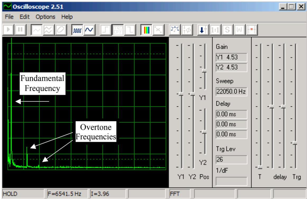
The frequency display for the same tube struck with the wooden end of the beater is shown below. Note the increased number of excited frequencies and the reduced fundamental height.
